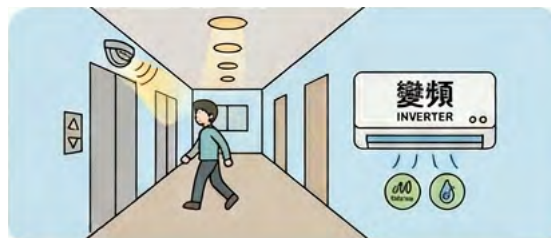
6. Automatic lighting system is installed in some areas, and the air conditioners are all installed with variable-frequency device.
